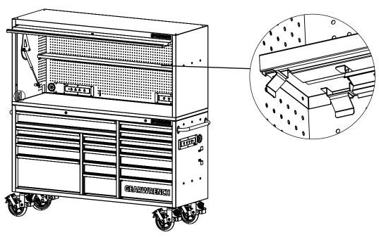
□ Use the Cable clips (EE) to attach the power cord from the LED light and route the wire along the backwall.
