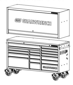
□ Use 8 pcs M6 x 48mm flange bolts (AA) to secure the Hutch along the sides and back to the Workbench. Tighten with a 8mm socket or wrench.
